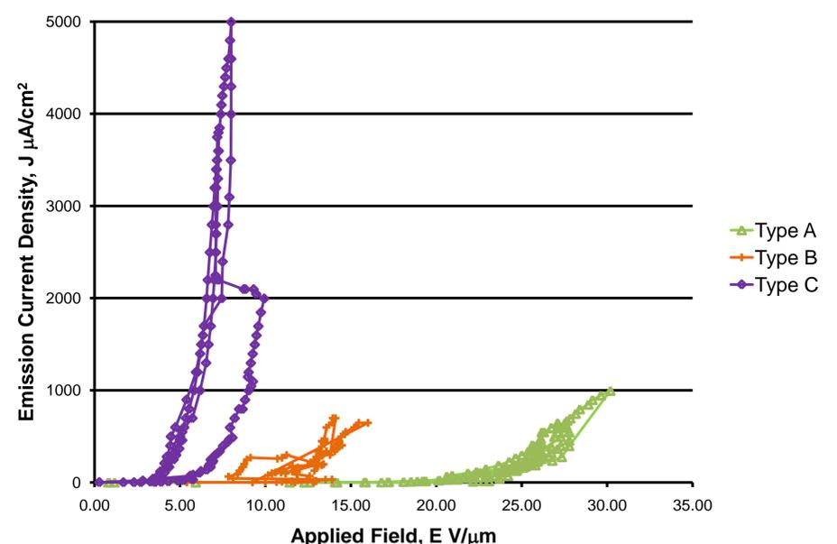
Fig 4: Plot of field emission performance of printed emitters
