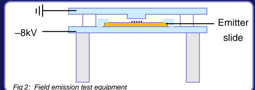
Fig 2: Field emission test equipment
