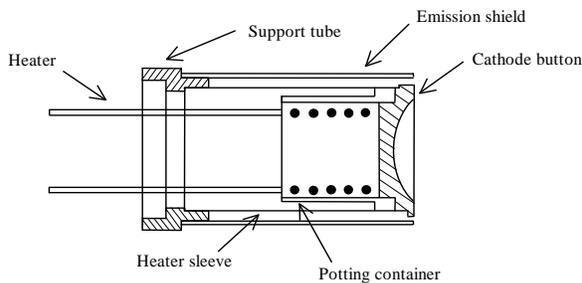
It was found sufficient to define cathode button as single 'lump' with a single temperature, potted heater wire as single lump at a single temperature, and a single 'lump' of potting at a single 'bulk' temperature. Other features included potting container, a two section cathode support sleeve, grids, support configuration to external HV seal, and an emission shield.
