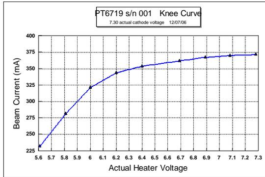
Figure6. Fast warm cathode knee curve - TMD
