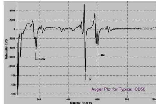
Figure2. Auger plot for typical CD cathode surface
