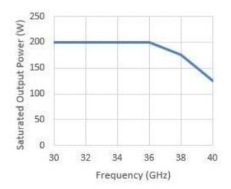
TMD's new line of Ka band compact MPMs is exemplified by the PTX8807 – operating over the 30-40 GHz range up to 200 W output power (100% max duty cycle).
