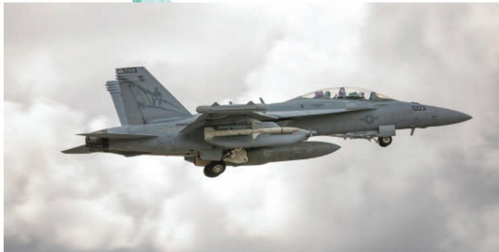
The EA-18G's ALQ-99 pods rely on TWTs to generate the power needed to perform its support jamming mission. DOD IMAGE
